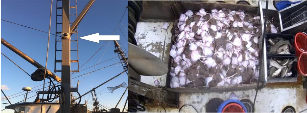
Figure 2: An overhead camera mounting which generates a broad, top-down view of sorting activities. Image provided by the NE groundfish audit project.
