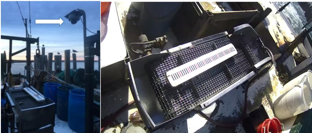
Figure 3: A fabricated mounting which generates a close, top down view of species ID and measuring. Image provided by the NE groundfish audit project.
