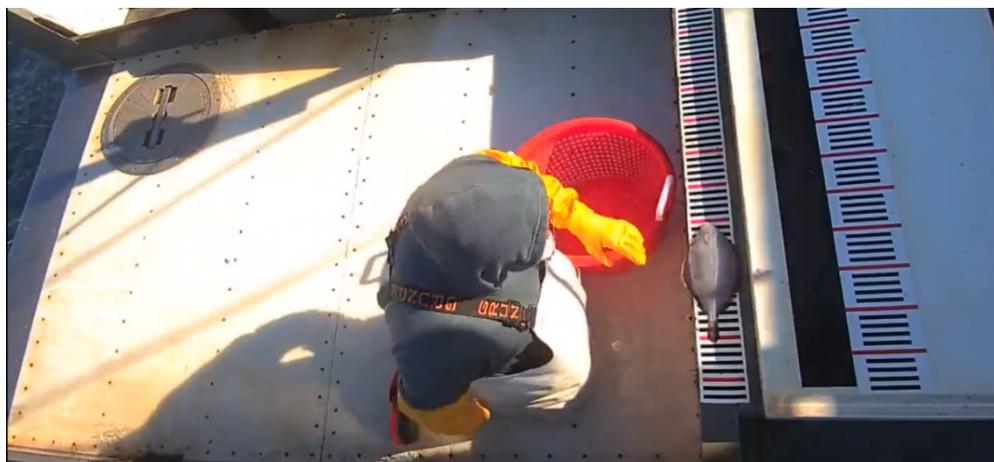
Figure 4: A fisherman measures discarded fish, using a measuring strip installed below the EM camera. The fish length, and calculated weight is captured during video review using this image. Image provided by the NE groundfish audit project.
