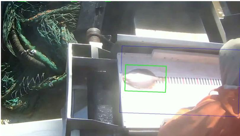
Figure 7: Image with a defined Region of Interest (ROI) in blue, as well as a localized fish in green. By restricting an algorithm's field of view to a specific ROI, performance is improved by excluding potential confusing scenery (e.g. background, totes with other fish in them, etc.). Image provided by the NE groundfish audit project.
