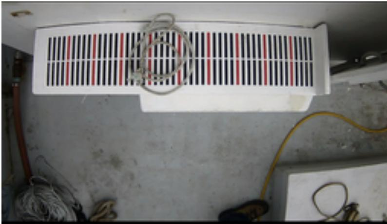
Figure 1: An example of a restricted field of view that captures only the measuring strip and its immediate surroundings. This tight view limits the amount of noise an algorithm needs to accommodate in the area surrounding the activity of interest. Image provided by the NE groundfish audit project.
